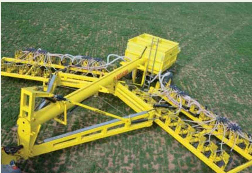
CLEVER: The Rotacon's folding system is unique and allows a transport width of just 3m. The main seeding bar folds in half, towards the front of the air seeder and then upwards, either side of the main frame.
