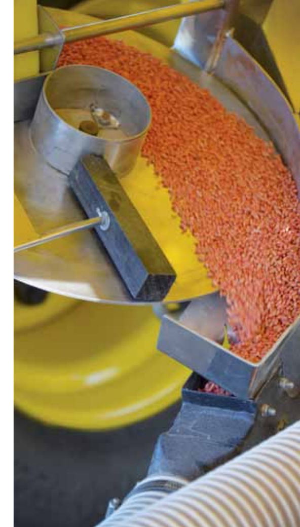
METERED OUT: The seed and fertiliser metering system is based on a rotating stainless steel disc.
